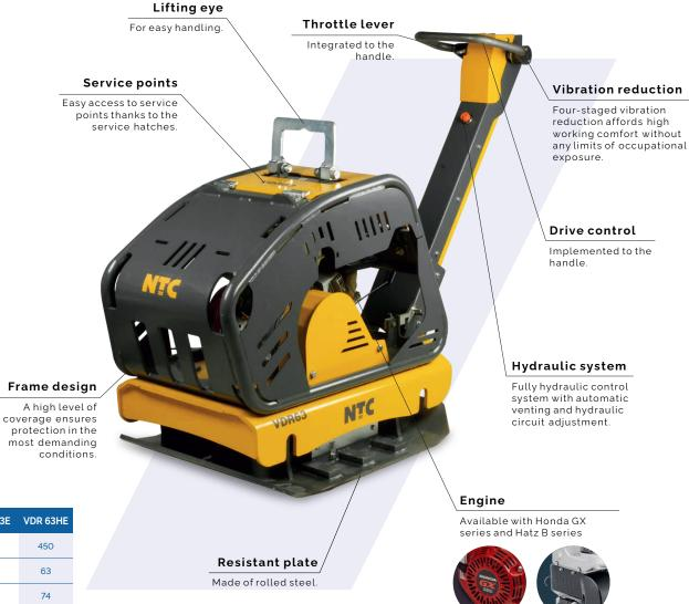
**TYPE VDR 52** VDR 52E VDR 52H VDR 52HE **VDR 63** VDR 63E VDR 63HE Weight | kg 355 360 415 340 370 430 450 Centrifugal force | kN 52 52 52 63 63 63 74 Frequency | Hz 75 75 75 75 74 74 **Engine manufacturer** Honda Honda Hatz Hatz Honda Honda Hatz **Engine type** GX 270 GX 270 1 B 30 1 B 30 GX 390 GX 390 1 B 50
